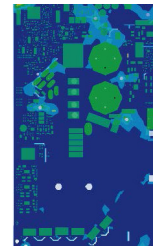
Ansys Sherlock displays strain distribution on PCBA from system simulation and solder joint or component cracking risk analysis. The components in green reveal there is no risk, a result achieved after several design iterations.
