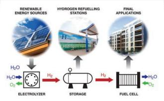
Hydrogen energy cycle: production, storage and transformation. Excess renewable energy production can be used by a water electrolyzer to produce hydrogen and oxygen. The hydrogen can be transported or stored in appropriate facilities, then when it is needed, hydrogen can be transformed into electricity using a fuel cell or it can be used as fuel in the mobility sector.
