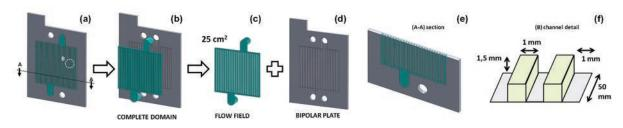
Geometry for the simulation model: (a) bipolar plate with the flow distribution channels; (b) complete domain; (c) parallel flow field; (d) bipolar plate; (e) section of the channels of the bipolar plate; (f) detailed dimensions of the channels
