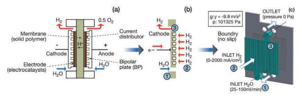
Model setup for the flow field in a PEM water electrolysis cell: (a) simplified scheme of a complete cell; (b) domain of the cathodic chamber considered in the model; (c) phenomena considered in the channels of the cathode
