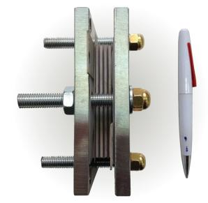
A PEM water electrolysis stack for hydrogen production with purity higher than 99.995%. The active area is 25 cm<sup>2</sup> and the maximum current density of 2,000 mA/cm<sup>2</sup>.
