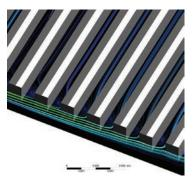
Streamlines at the closest part of the bipolar plate to the channel inflow at 500 mA/cm<sup>2</sup> and 100 mL/min. In some channels, when the flow rate is high, vorticity phenomena may occur. This limits the water flow in each channel so that the hydrogen generated in the cell accumulates, reducing the efficiency of the process.
