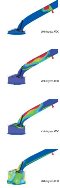
Cryogenic port injection plots show hydrogen mass fraction and motion of hydrogen as it flows into the cylinder during the intake stroke of the engine. As the intake valve opens and the piston drops down away from the valves, the piston motion draws the fuel air mixture in through the intake port.
