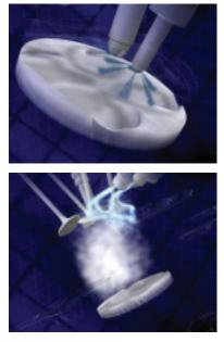
Two injection methods examined under the HylCE project: (top) direct injection of high-pressure hydrogen and (bottom) port injection using cryogenic hydrogen Image © BMW Group
